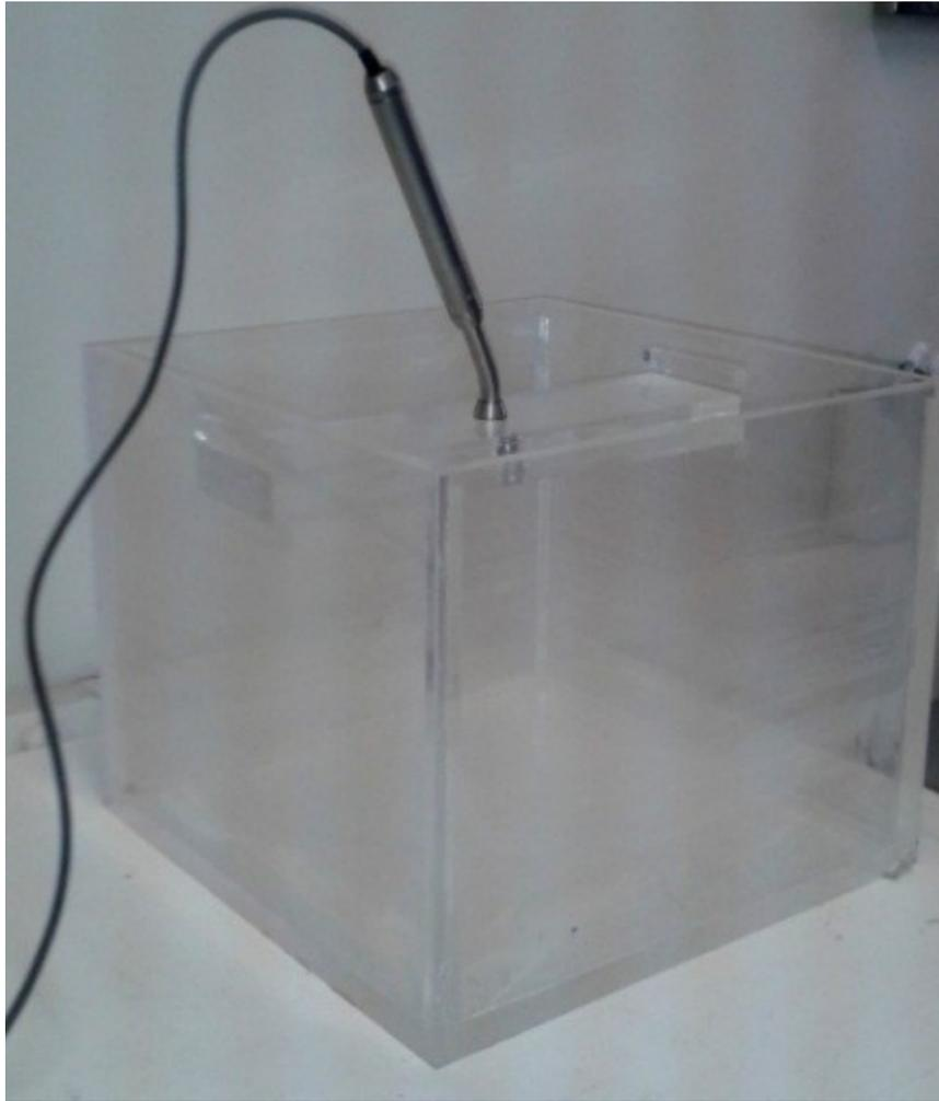
**Figure 4.** The measurement set-up for the evaluation of the spatial resolution and sensitivity in a scatter medium using a water bath with the size of 25 cm × 25 cm × 20 cm.
