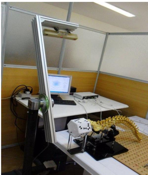
**Figure 1.** Illustration of the proposed hybrid system. The video-optical tracker is attached directly on the Pseudo C-arm Simulator.
