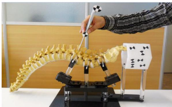
**Figure 3.** A “six-facet” reference marker is fixed on the spine phantom along with an example tracking tool.
