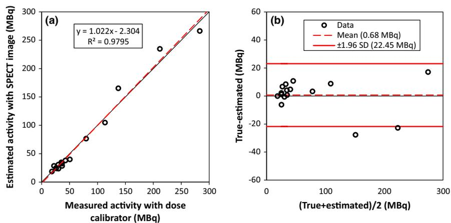
**FIG. 4.** (a) Comparing point source activities measured with the dose calibrator and estimated from reconstructed images, (b) Bland-Altman plot of these data.
